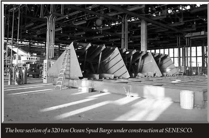
The bow section of a 320 ton Ocean Spud Barge under construction at SENESCO.
