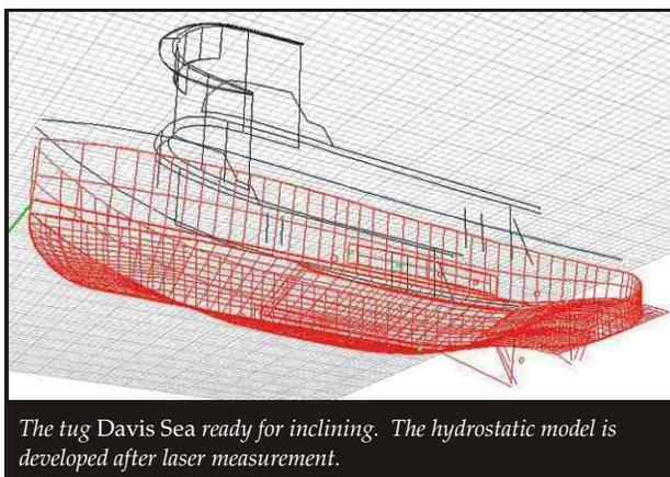
The tug *Davis Sea* ready for inclining. The hydrostatic model is developed after laser measurement.
