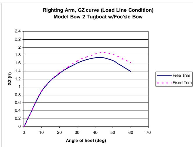
Fig. 26 (Loaded Condition Righting Arm Curves)
