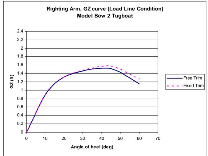
Fig. 22 (Loaded Condition Righting Arm Curves)
