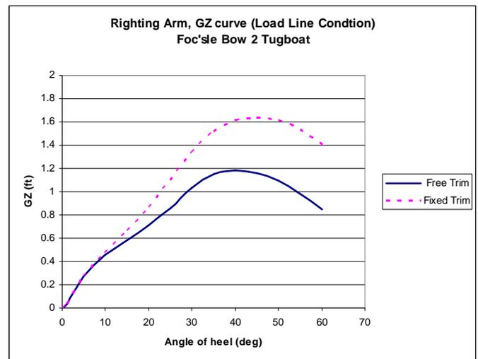
Fig. 9 Loaded Condition Righting Arm Curves
