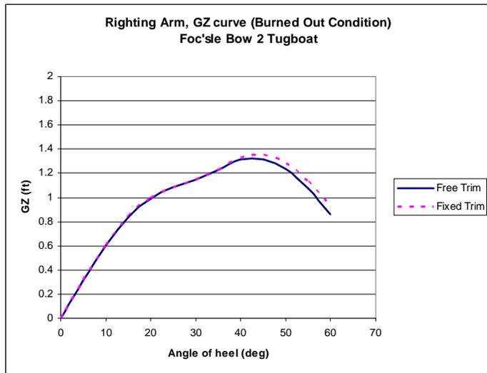
Fig. 7 Burned Out Condition Righting Arm Curves
