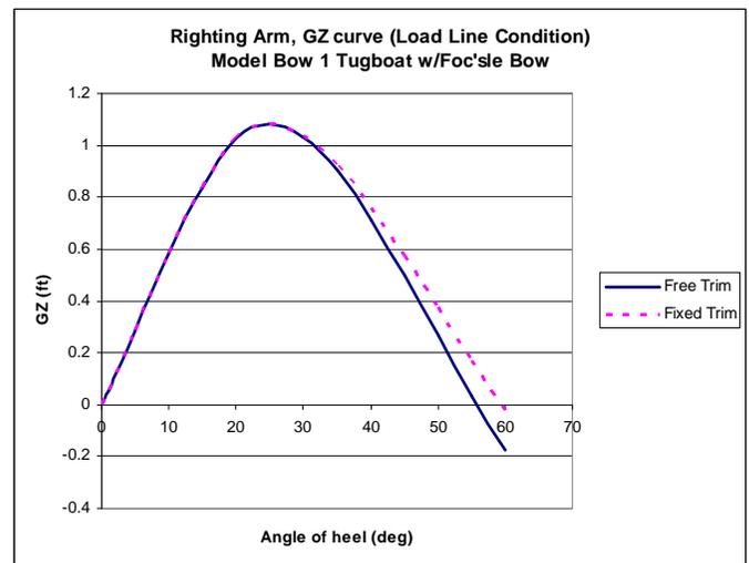
Fig. 18 Loaded Condition Righting Arm Curves
