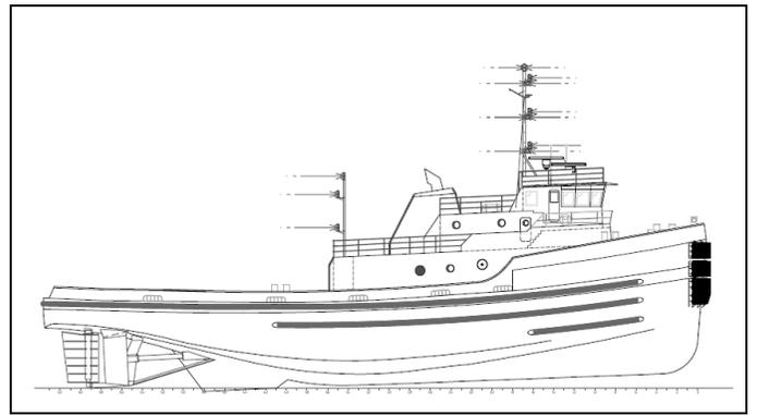
Fig. 23 Model Bow Tugboat 2, w/Foc'sle Bow.
