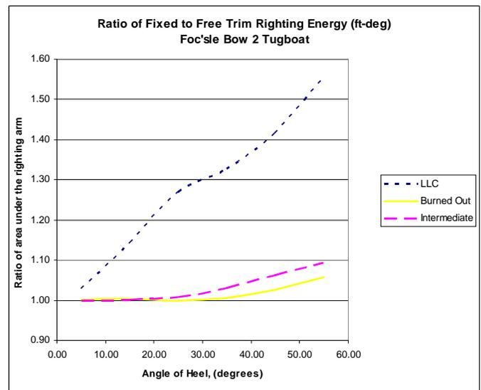
Fig.10 Ratio of Righting Arm Curves
