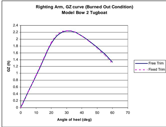
Fig. 20 (Burned Out Condition Righting Arm Curves)
