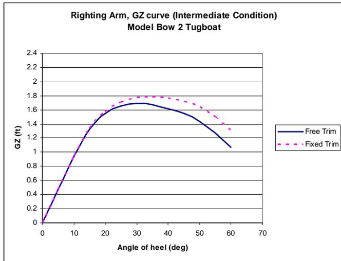
Fig. 21 (Intermediate Condition Righting Arm Curves)
