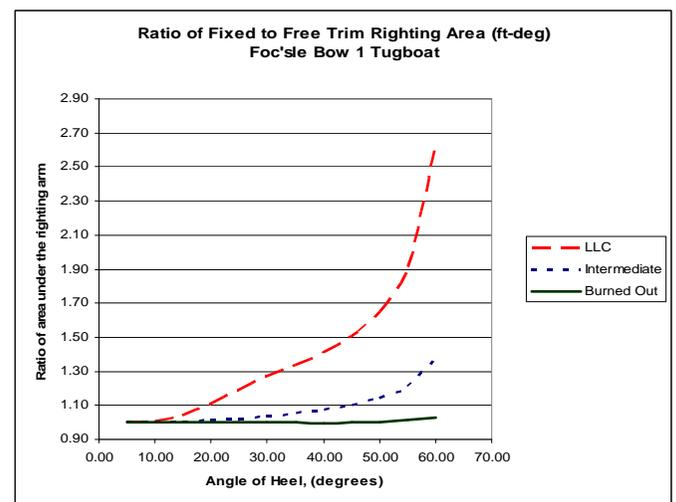
Fig.5 Ratio of Righting Arm Curves.
