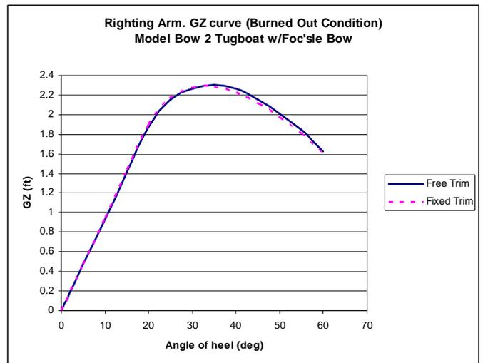
Fig. 24 (Burned Out Condition Righting Arm Curves)
