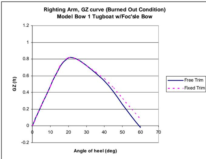
Fig. 16 Burned Out Condition Righting Arm Curves
