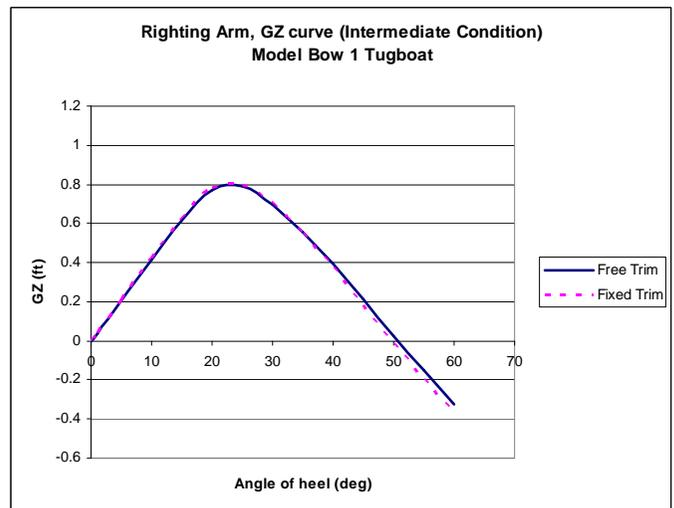
Fig. 13 Intermediate Condition Righting Arm Curves
