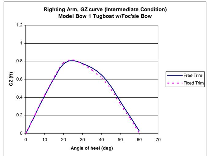
Fig. 17 Intermediate Condition Righting Arm Curves
