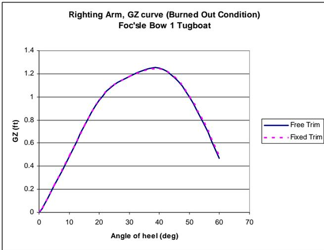
Fig. 2 Burned Out Condition Righting Arm Curves
