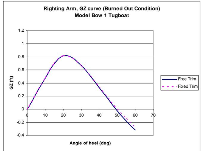
Fig. 12 Burned Out Condition Righting Arm Curves
