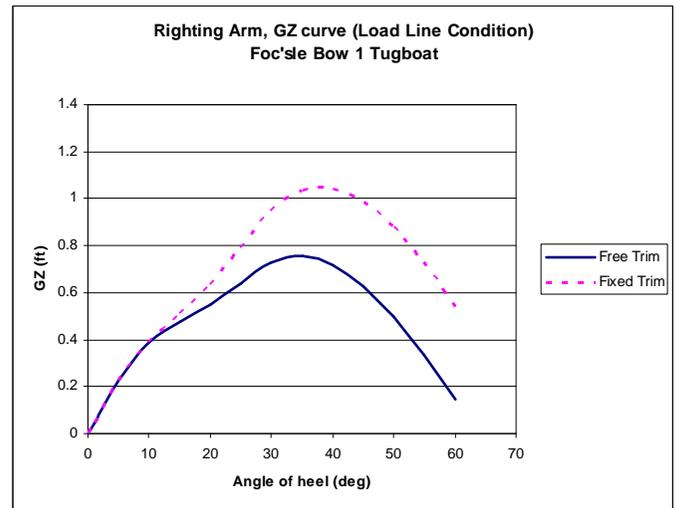
Fig. 4 Loaded Condition Righting Arm Curves.
