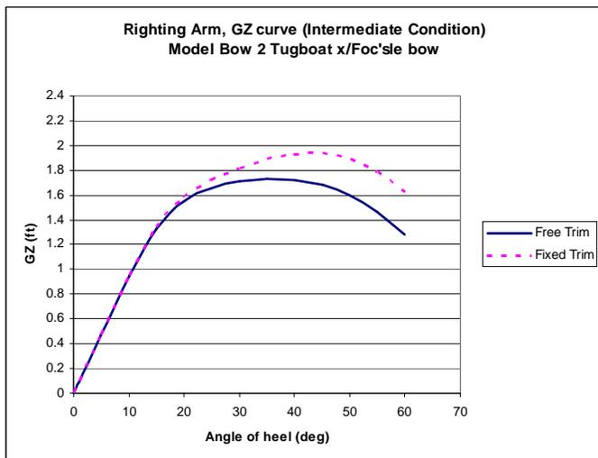
Fig. 25 (Intermediate Condition Righting Arm Curves)
