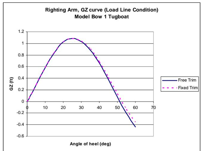
Fig. 14 Loaded Condition Righting Arm Curves
