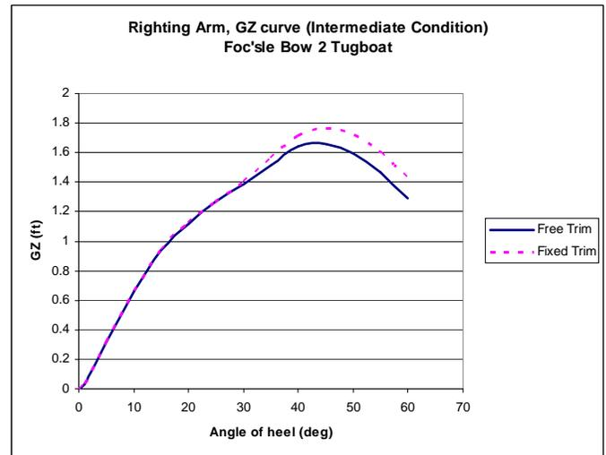
Fig. 8 Intermediate Condition Righting Arm Curves
