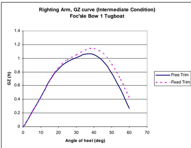
Fig. 3 Intermediate Condition Righting Arm Curves.
