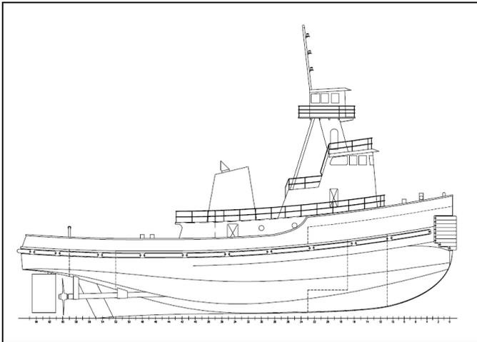
Fig.15 Model Bow 1 Tugboat w/Foc'sle Bow
